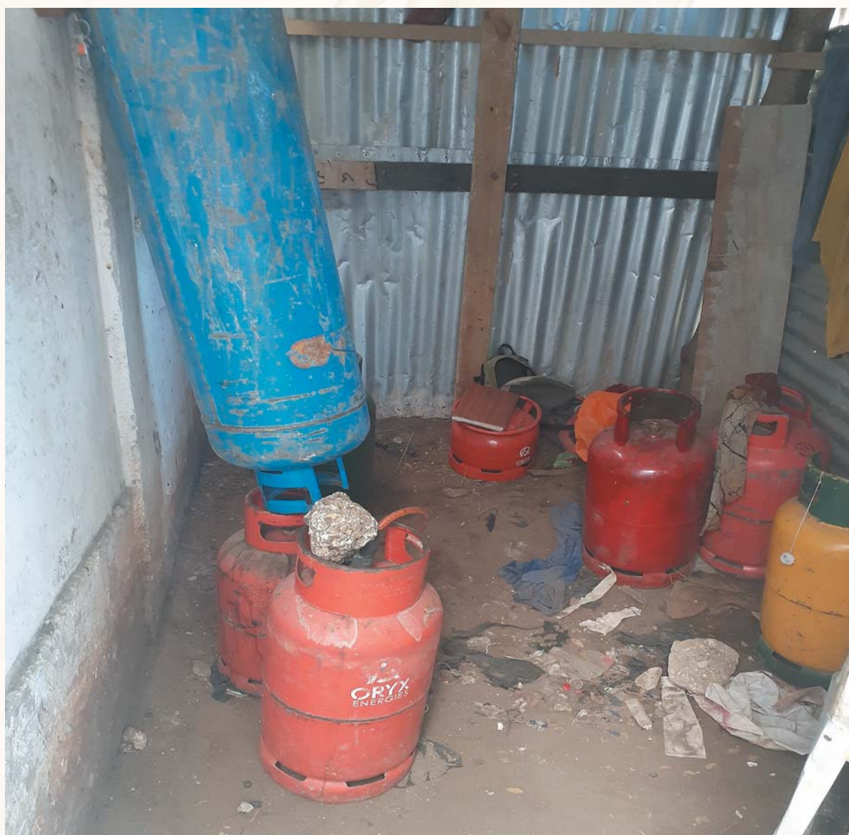
Figure 23: Illegal LPG refilling operation at Nkurumah Street, Kariakoo in Dar es Salaam
