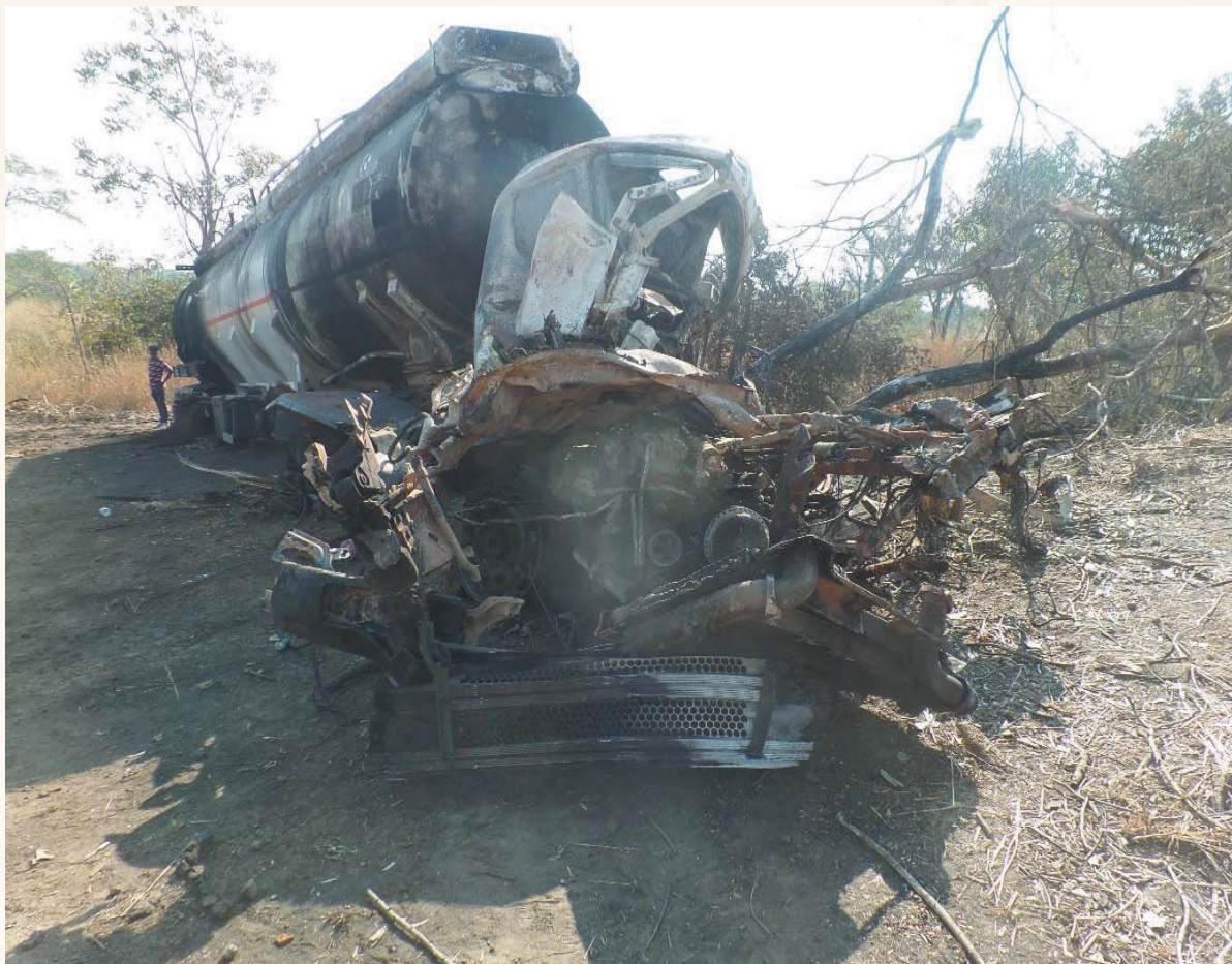
Figure 30: A driver cabin of truck no. T243 BCU / T685 DCV that was completely damaged
